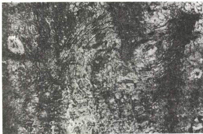
Fig. 4. Concentric pattern of diffusion bands in disaggregated limestones. Guira de Melena, Cuba.
